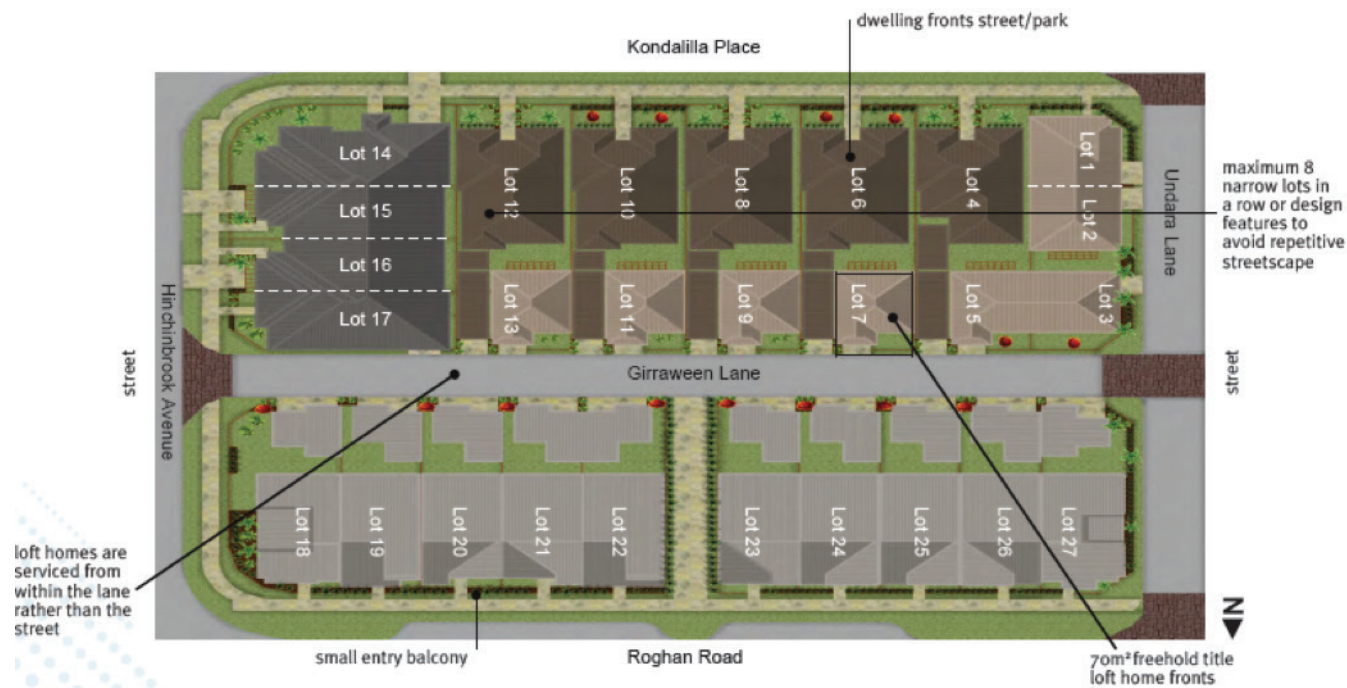
Figure 5.18 - Servicing small freehold dwellings off a rear laneway (Image supplied courtesy of Ausbuild)
